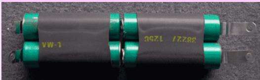
Figure 3 - NiCad Cells in series and wrapped
